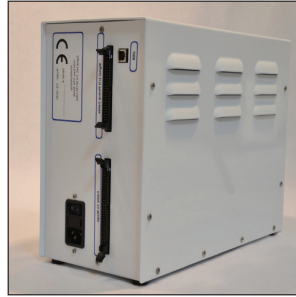
Front and back views of the LS-AFM Ebox showing indicator lights and connectors for ribbon cables and USB
